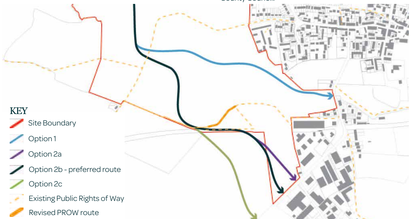
Figure 46: Central Residential Boulevard alignment options considered
