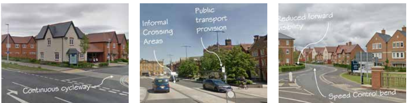
Figure 36: Examples of typical intervention strategies to discourage the use of the Central Boulevard as a 'rat-run'
